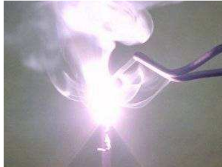
A light, silvery-white, moderately hard, metallic element that in ribbon or powder form burns with a brilliant white flame. Magnesium is the second lightest member of the alkaline earth metals (after beryllium). Magnesium was formerly used to make flash bulbs in photography.
