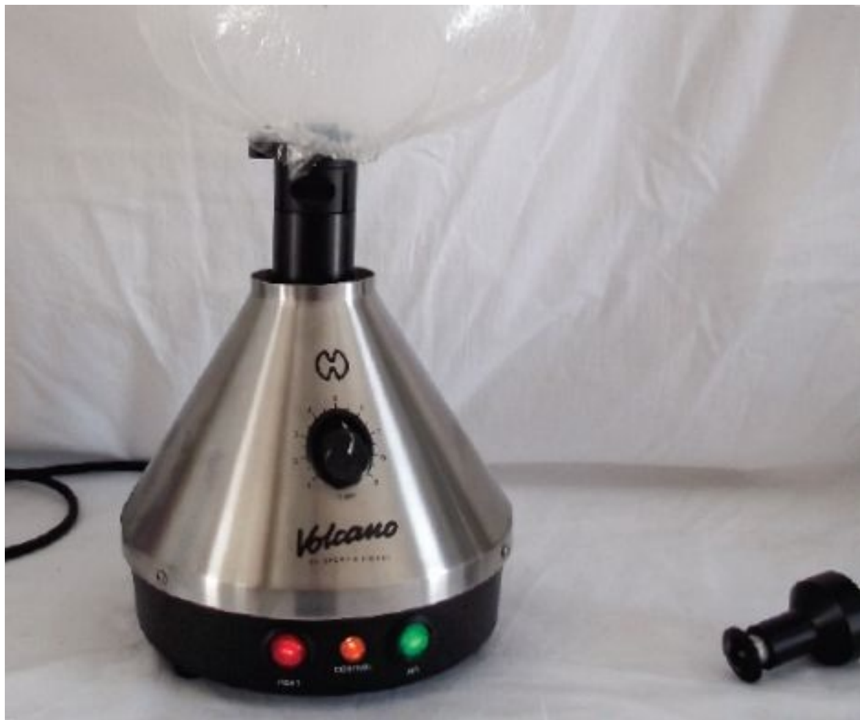
Volcano vaporizer. The vapor is collected in the bag for inhaling.
